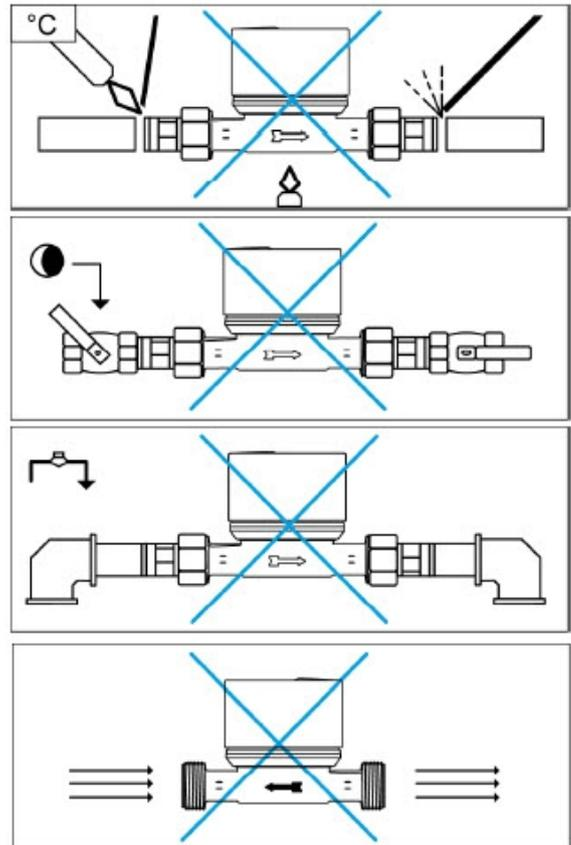
Figure 1: Examples of mounting a water meter.
