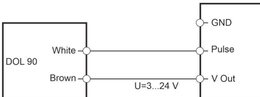
Figure 2: Example of connection
